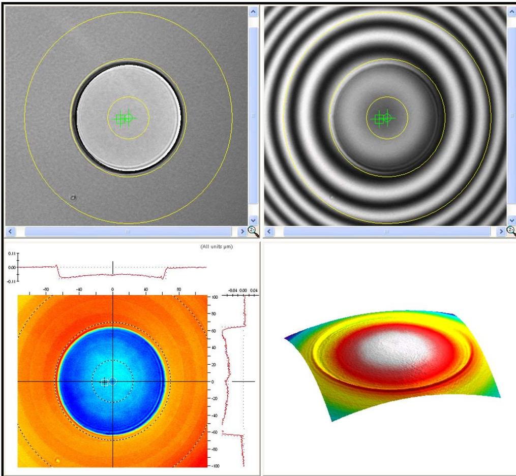
**Figure 4 – End Face Interferometry Check**
